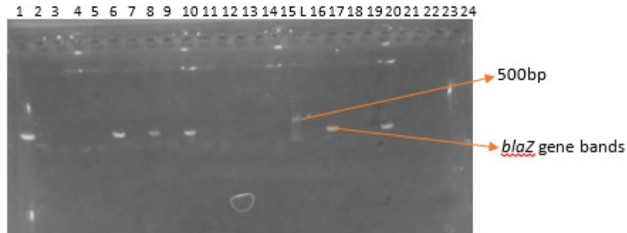
Fig. 2: Agarose gel electrophoresis showing the amplified blaZ gene bands. Lanes 1,6,8,10,17 and 20 showing the amplified bands at 300bp while lane L represents the 1000bp molecular ladder
